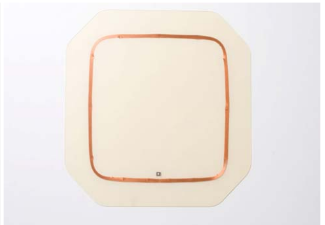
Photo 4: TGL2, Thin-Laminated RFTag (Toppan Printing Co., Ltd.)
